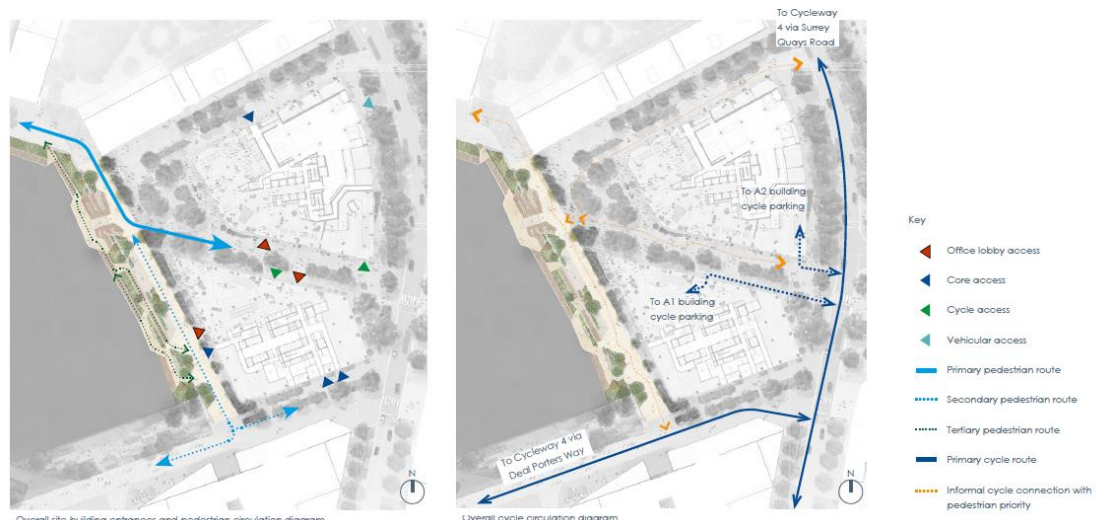
Image above: Overall site building entrances and pedestrian circulation diagram [right] and overall cycle circulation diagram [left]
